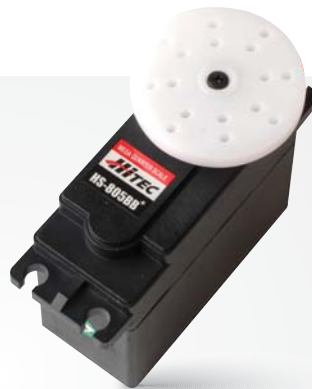
HS-805BB MEGA QUARTER SCALE 4.8 V Torque : 19.8 kg.cm 4.8 V Speed : 0.19 sec/60° 6.0 V Torque : 24.7 kg.cm 6.0 V Speed : 0.14 sec/60° Dimensions : 66 x 30 x 57.6 mm Weight : 110 g Stock# 31805S
